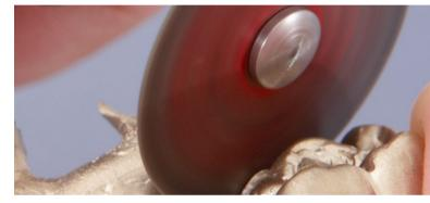
Flexible and robust, doubly glass fiber reinforced separating disc for precious and non-precious metal.
